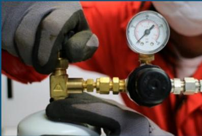
The EMT Smartfill CTU can connect to any standard SF6 gas cylinder utilising quick connect adaptors
