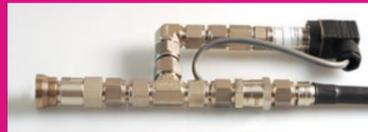
The Smartfill CTU filling outlet hose has an inbuilt pressure sensor to directly measure the SF6 pressure within the compartment. A non-return valve is also built into the hose to prevent venting of compartment gas
