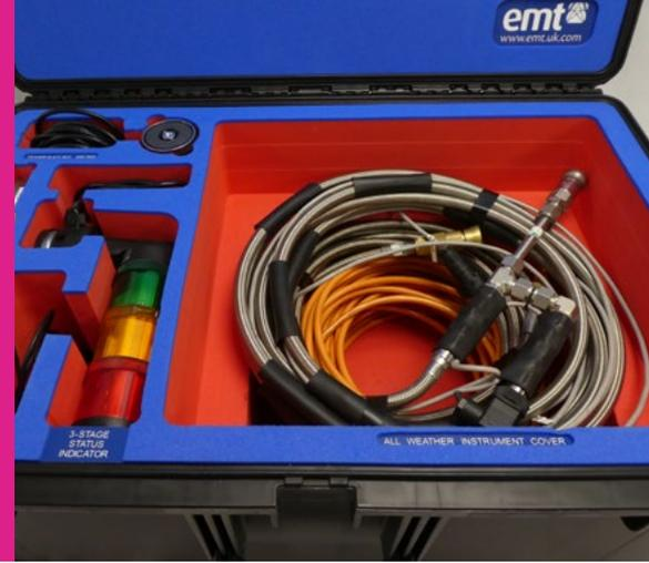
The EMT Smartfill advanced accessory kit is designed to ensure engineers always have the equipment they need to perform a fill, top-up or continuous top up of an SF6 compartment.
